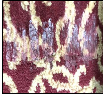
Two pictures above show melted yarn from dry friction.
