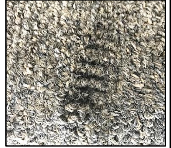
Two pictures above show melted yarn from dry friction.
